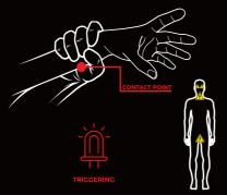
CONTACT: Grab the assailant, avoiding the areas considered dangerous (eyes/jugular/testicles). Upon contact of the glove with the assailant, the contact button located in the middle of the palm of the hand will trigger the electrical impulse (Triggering).
